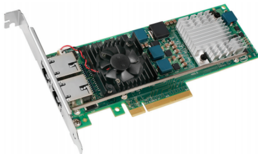
Fig. 6.19 – Scheda Intel X520-T2 (Dual Port 10GBASE-T)
